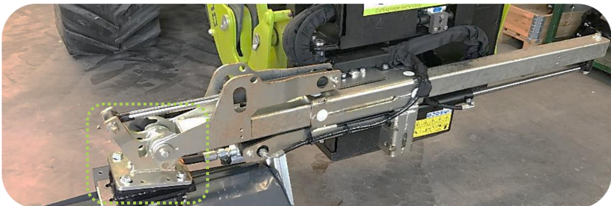
Assembly example of attachment tool on PUMA Tele Multi Carrier
