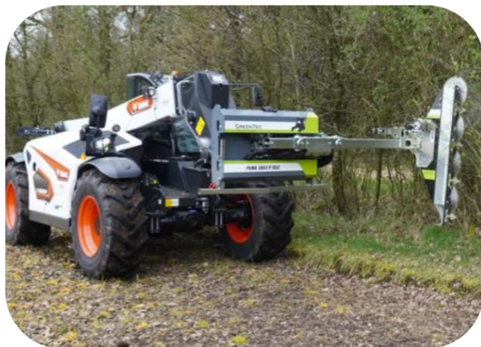
PUMA 2803 Tele Multi Carrier with LRS 1602 Quadsaw in vertical position
