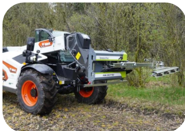
PUMA 2803 Tele Multi Carrier with LRS 1602 Quadsaw in horizontal position
