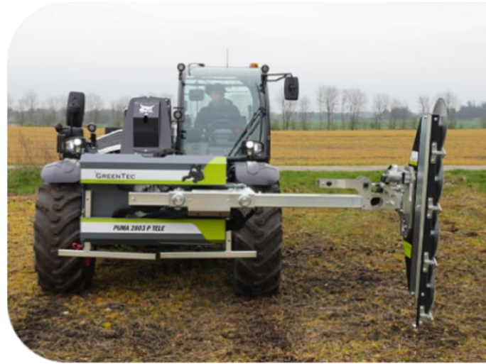
PUMA 2803 Tele Multi Carrier in use with LRS1602 Quadsaw
