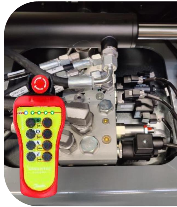
Oil flow divider w. e-control: PUMA 2803 Tele Multi Carrier
