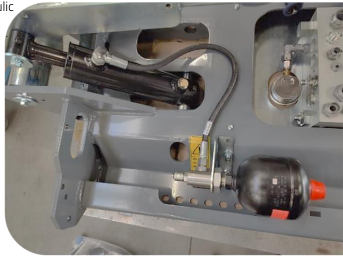
Accumulator connected to impact cylinder
