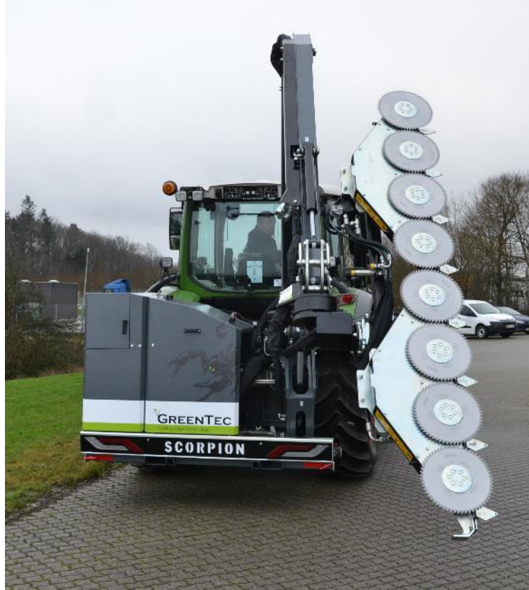
LRS 2002: 4.0 m working width / Ø 16 cm
